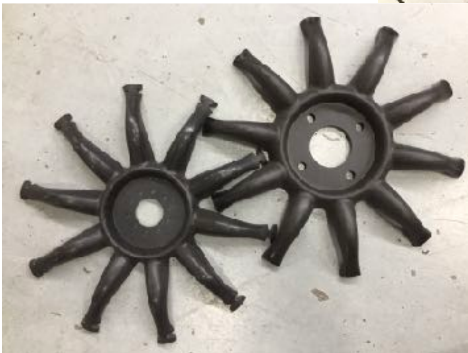
Left; CBW1 Hybrid with 5/10 bolts on 60 mm circle. Right; CBW5 Hybrid 50 mm rim with 4/100mm.
