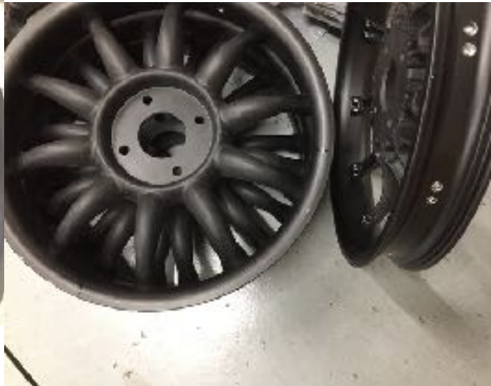
Left; CBW1 Hybrid with 5/10 bolts on 60 mm circle. Right; CBW5 Hybrid 50 mm rim with 4/100mm.
